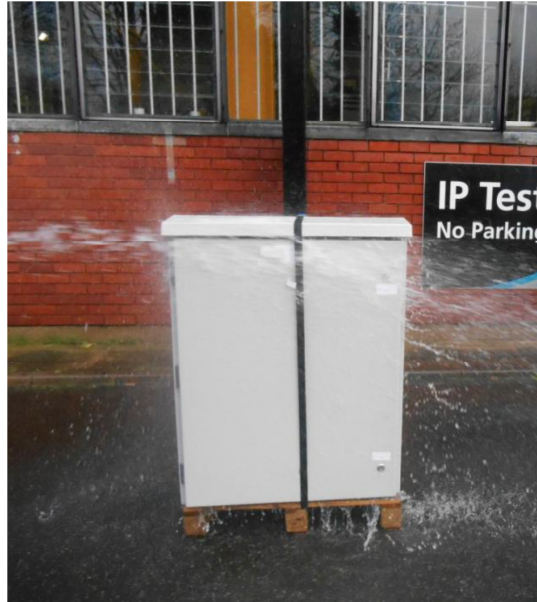
FIGURE 1. SPECIMEN S2 UNDERGOING IPX5 WATER JETTING
