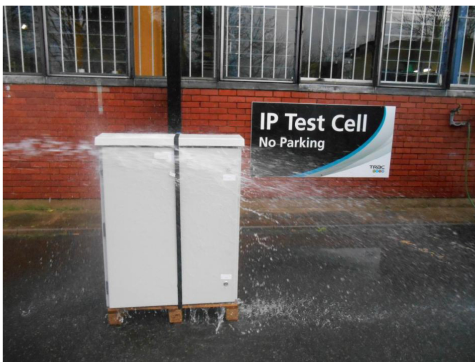
FIGURE 1: SPECIMEN UNDERGOING IPX6 POWERFUL WATER JETTING
